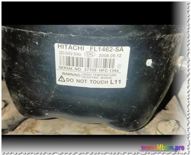
Compressor, Hitachi, R134a, (série R012), FL1462-SA, HITACHI Brand, (Made in Thailand), T/5 Hp, 160w, Fl 0739 (90 Watts), Fl 0847 (105 Watts), Fl 1152 (125 Watts), Fl 1257 (150 Watts), Fl 1462 165 Watts), Fl 1675 (185 Watts), Fl 1888 (250 Watts)
