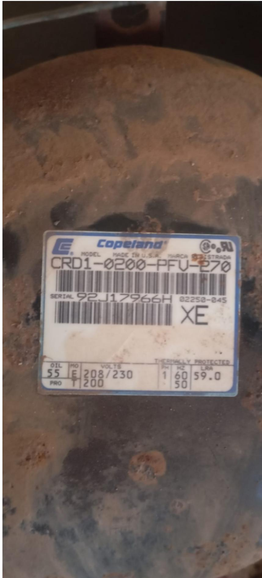
Copeland, CRD1-0200, 2 HP, 208-230V, 1 PH, 24,500 BTU, R22, R407C, Hermetic (Reciprocating) Compressor Replacement • OEM Upgraded Copeland Compressor
